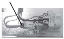
When doing a hard-wire installation, you must remove the supplied power cord.
